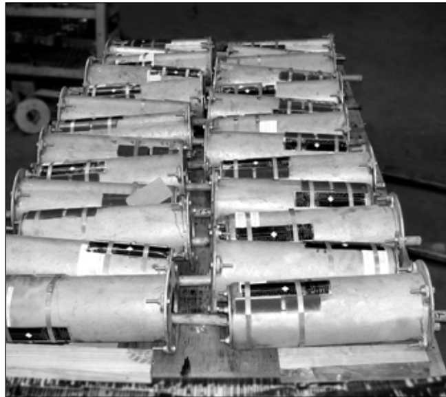
PTP-4 TYPE A VARIABLE SPRINGS WITH A DOWNWARD TRAVEL OF 1.375"
